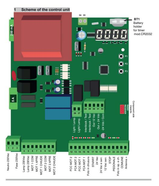
Normally the red led in the inputs OLS - CLS - STOP - FOTO are always lit on.
