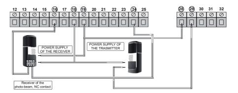
The TEST of the photo-beam works only if the photo-beams are installed properly. The control unit will check all connections before opening!
