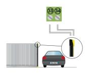
Connection of the ALT control: Stops the automation and activates an inversion of direction for approximately 1.5 seconds.
