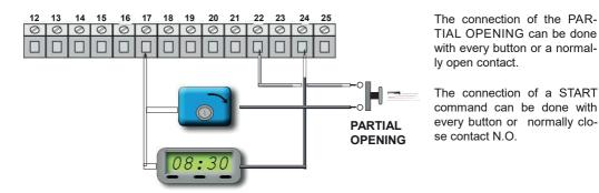
If more devices are available they should be connected in serial. Connect a timer in the terminal board no. 17 and 22 to programm the opening time of the gate. The timer contact should be no. (normally open) and it should be closed when the gate is opening. If the it is available the connection in the terminal board no.17, connect it in serial
