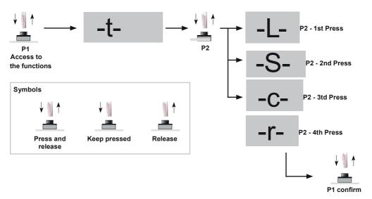
Confirm with P1 in the set up R and you can go to the "subfunction", choosing with the buttons P2 and P3 and then confirm with P1. Now we are in the function R01. R02. R...
