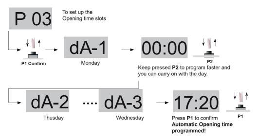
Once the opening hour time has been confirmed, the display starts flashing. Press **P2** to programm the hour and the day. The set up starts from the last programmed hour.
