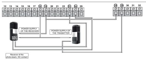
The TEST of the photo-beam works only if the photo-beams are installed properly. The control unit will check all connections before opening!
